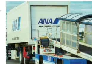
Belt loader for loading luggage on aircraft
