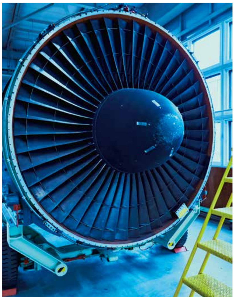
▶ Turbo fan engine that was mounted on the Boeing 747, commonly known as the Jumbo Jet.
