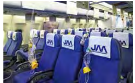
▶ Mock-up seating equipped with oxygen masks that activate during rapid decompression
